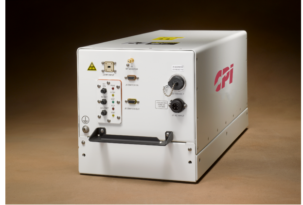
CPI 750 W air cooled Ka-band TWTA, provides up to 350 or 340 watts of linear power at the flange
